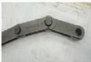
Photo 4 - Mode of failure (ST028 - 50,000lbs)
